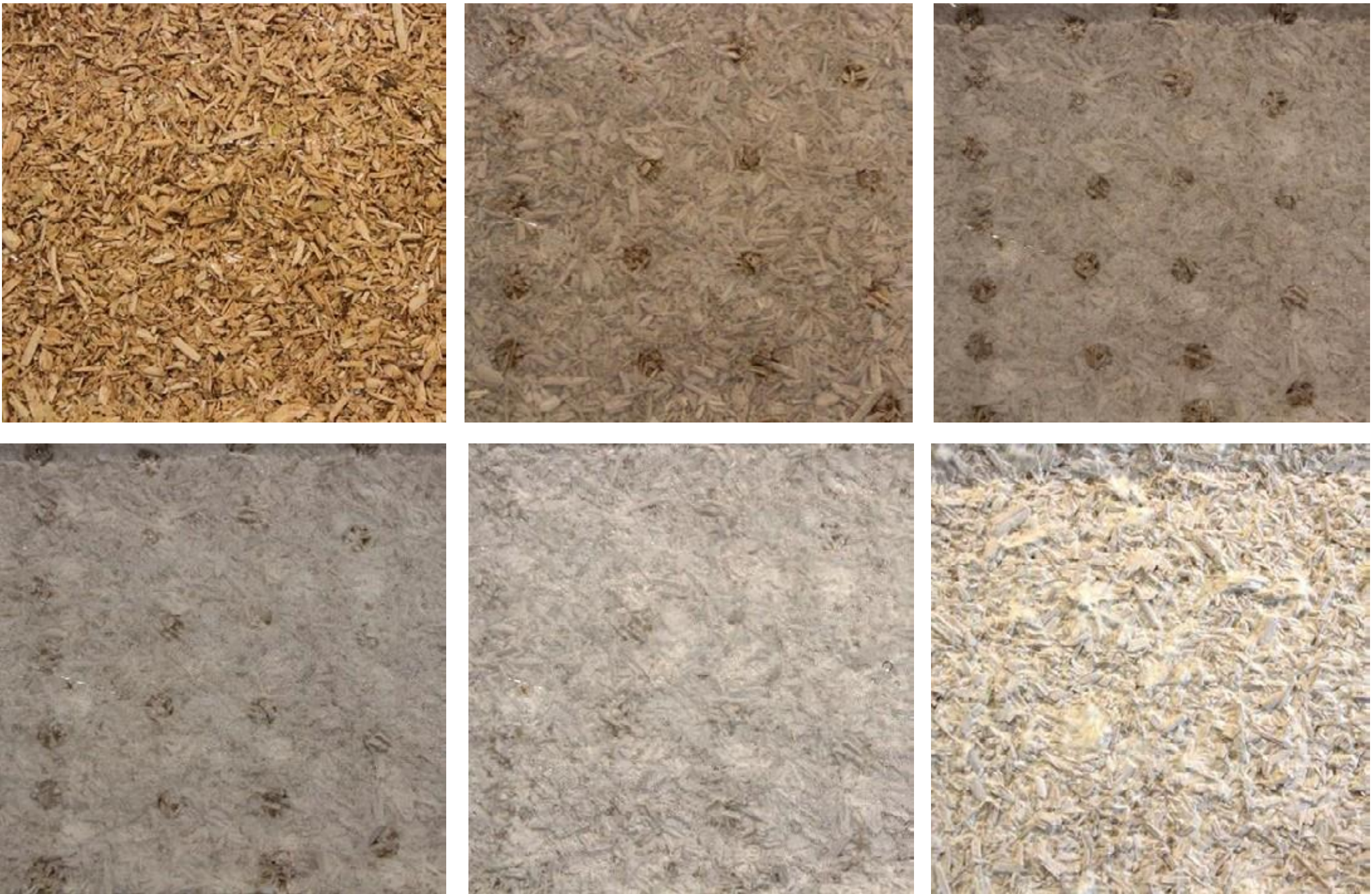
(above) Growth Day 1-6 - Mycelium Lemon Peel Boards (right) 3-Point Beng Mechanical Test Photo Credit: I. Ridwana
