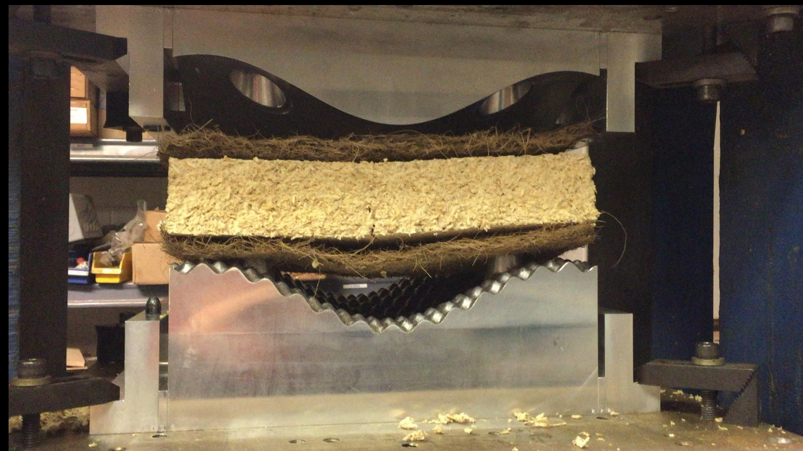
Pressing of Coconut AMBIS Module at e2e Materials Credit: Mae-ling Lokko
